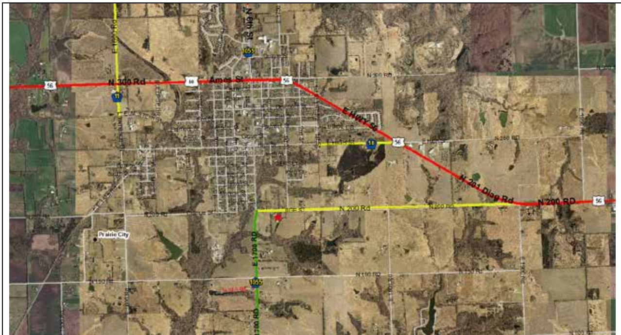
Figure 4: Map of area with street classifications: principal arterials shown in red, minor arterials in green, and minor collectors in yellow. Subject property marked with a star.
