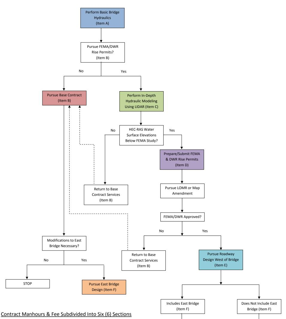
**Item A** – Conceptual Phase; Perform Traditional Bridge Hydraulics. Compare Water Surface Elevations to Existing FEMA Flood Insurance Study to Determine if Pursuit of In-Depth Hydraulic Model is Warranted. If WSE Lower than Study, Pursue More In-Depth Model. If WSE Higher, Evaluate Longer Bridge to Achieve a No-Rise Situation.
